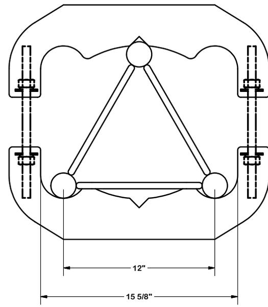
BCAM-HDLL on #12 Truss Leg
