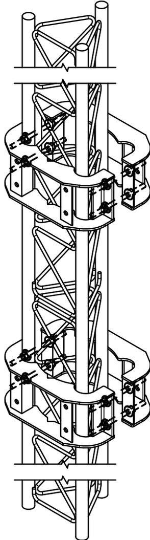
BCAM-HDLL on #12 Truss Leg
